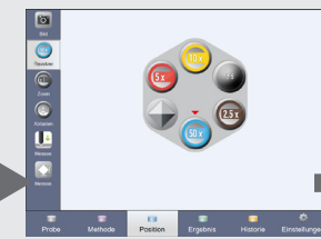
The turret shows the currently swiveled-in objective or indenter
